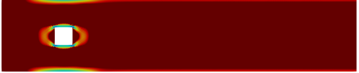
(b) Effective viscosity for a power-law fluid with r = 1.3 and \nu = 0.5 .
